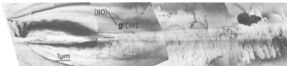
Figure 2 Another type of the plastic zone formed in polycrystalline nickel. The plastic zone is broad and the dislocations in the plastic zone are perfect dislocations.
